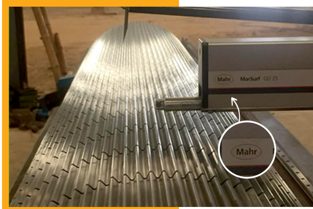
Flute profile testing on MAHR (German make) Equipment
